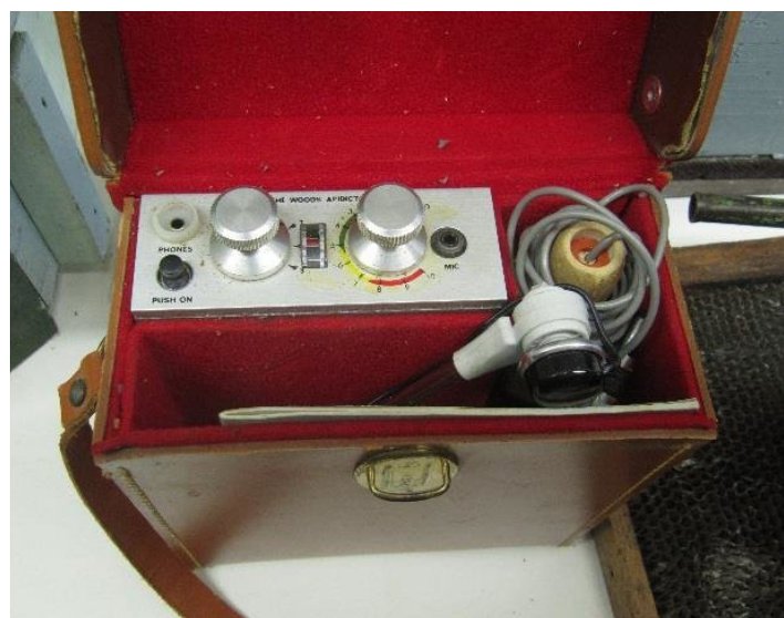
The Apidictor, invented by Edward Woods in the 1950s for listening in to beehives as a form of swarm warning. The device didn’t take off globally, but the use of devices to predict hive states is becoming increasingly common explains Dave Black.
