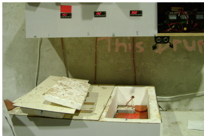
Ashburton Apiaries incubators made out of shower lining and polystyrene for cells at day eight. They have three and each compartment holds 144 cells.
