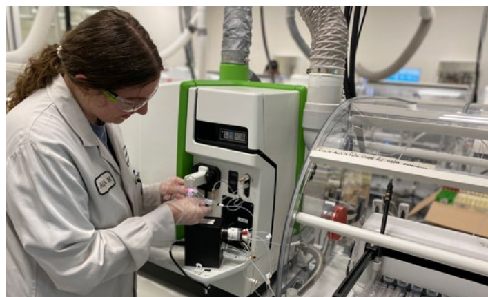
A Hill Labs technician sets up the ICP-MS machine to run honey samples to detect heavy metal levels.
