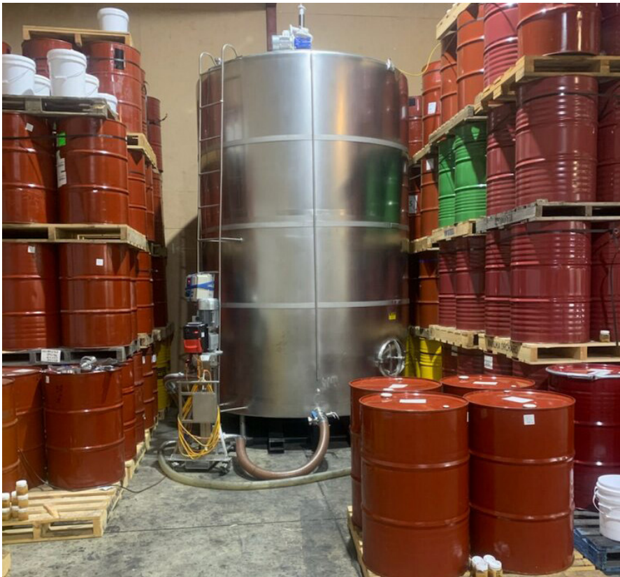
Mānuka Orchard's 20-tonne blending tank in the Bay of Plenty, which can help beekeepers add value to their honey stocks.
